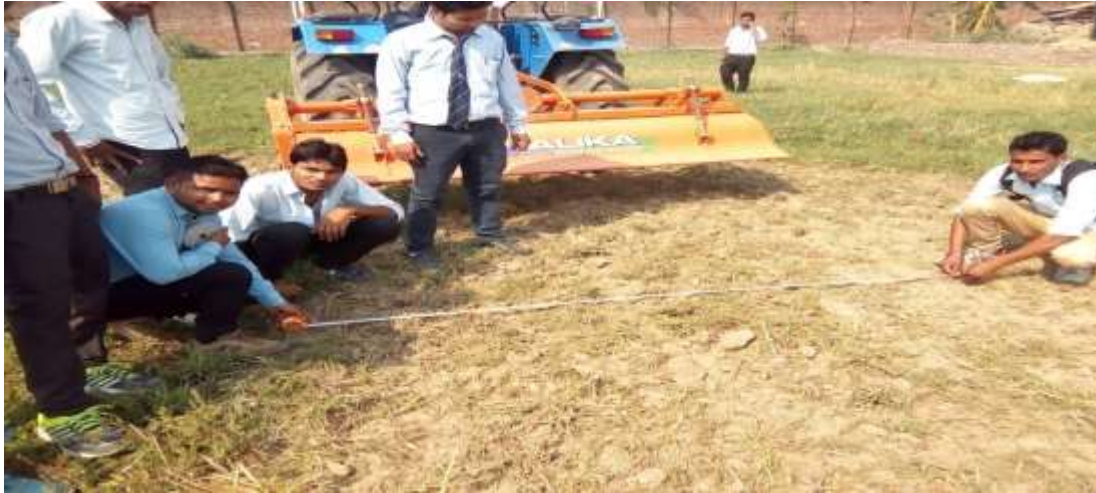
Figure1: The Measurement of Actual Working Width of Rotavator
